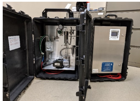
Figure 1: GreenPath's Field Vent Gas Spectrometer
